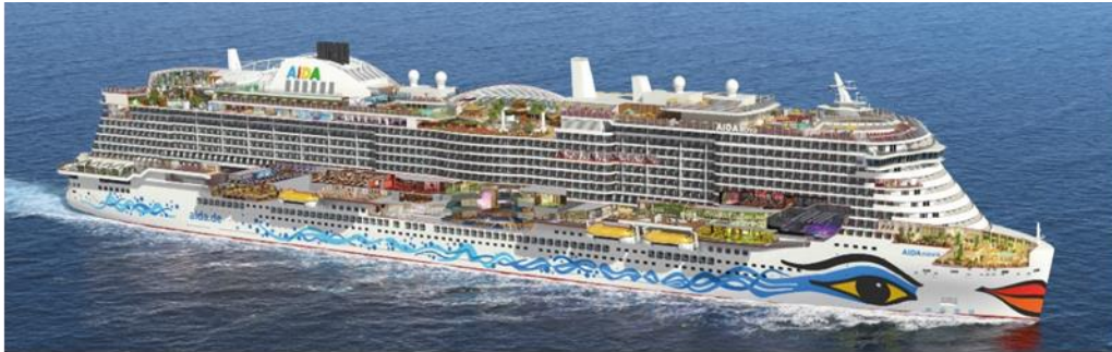
AIDAnova: world's first LNG cruise ship, ordered in 2015, delivered in Dec. 2018
