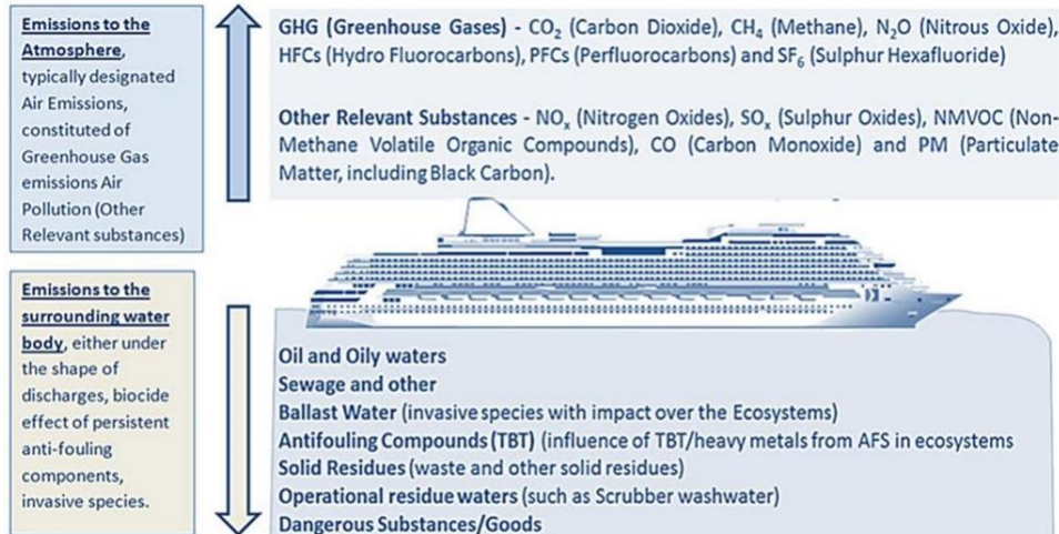
Figure 4.1 Pollutant emissions to the atmosphere and water body from a generic ship. Source: (EMSA)
