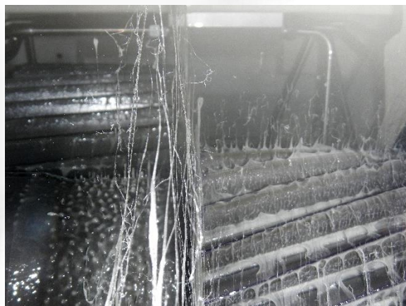
Example testing of new gearbox lubricants
